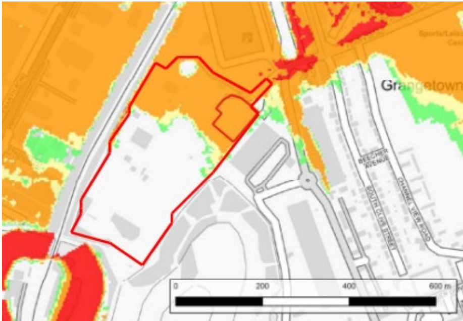
Figure 4 – 1 in 1000+CC Flood Extent
